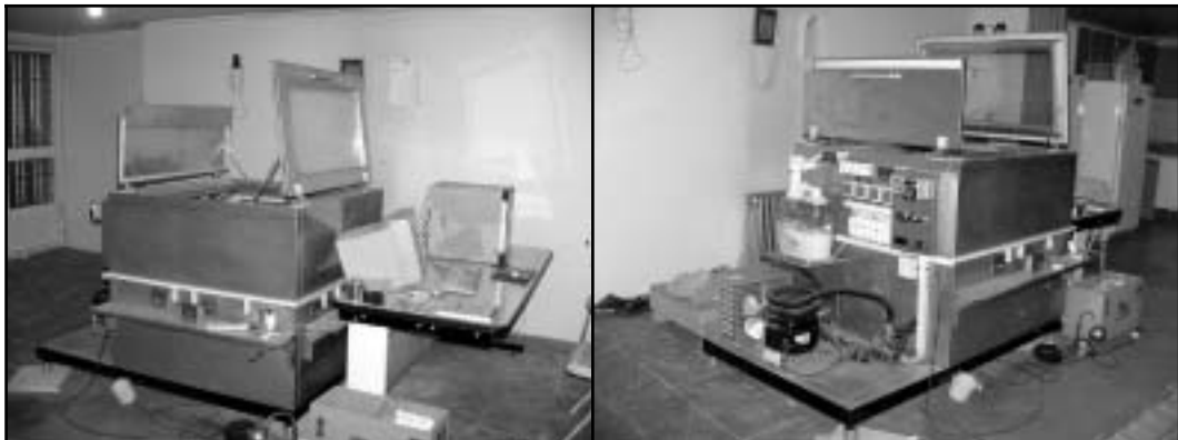
Figure (2): A Typical Photo of the Simulator Apparatus to Measure Carpet Compression Creep Behavior
